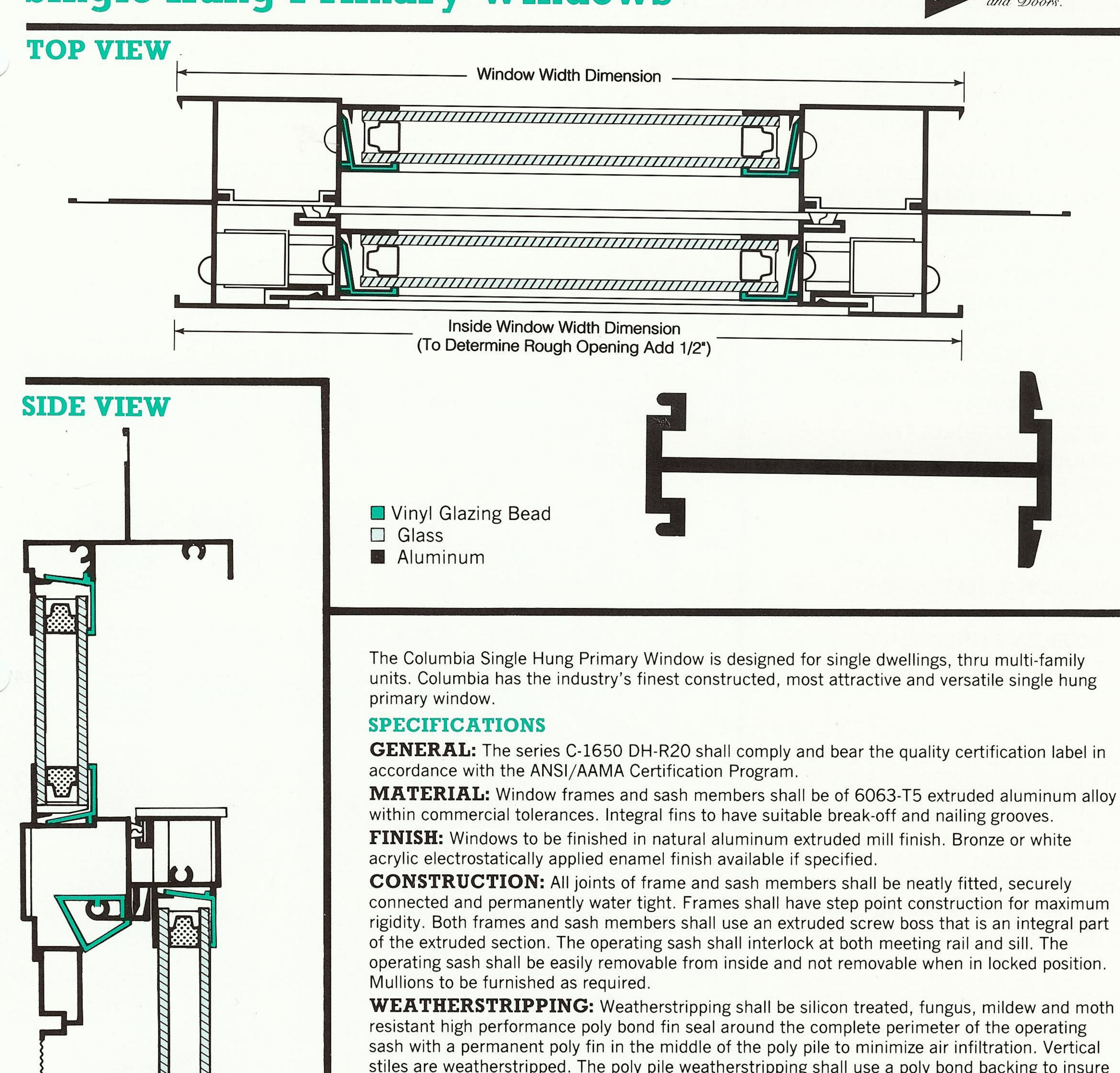
WEATHERSTRIPPING: Weatherstripping shall be silicon treated, fungus, mildew and moth sash with a permanent poly fin in the middle of the poly pile to minimize air infiltration. Vertical stiles are weatherstripped. The poly pile weatherstripping shall use a poly bond backing to insure against shrinkage. Bottom sash rail is also furnished with a vinyl seal for double protection.
